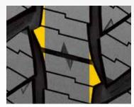
A zig zag block edge design increases traction in dry, muddy and snowy conditions.
