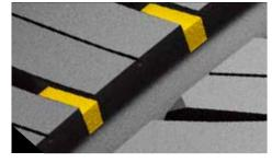
Tie bars that connect the shoulder blocks reinforce the stiffness of the shoulder tread for maximum cornering grip and minimized irregular wear.
