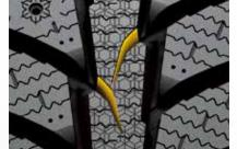
A claw-shaped 3D edge design in the tire's center tread blocks helps to improve traction performance on snowy and icy roads.
