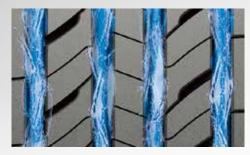
Four wide, straight tread grooves provide efficient water drainage in wet conditions for improved vehicle stability.
